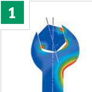
Load zones in standard-quality spanners
