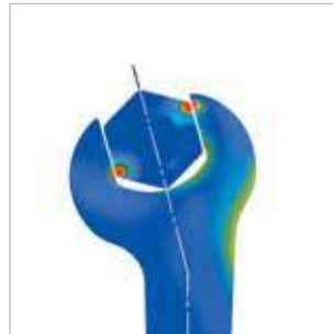
Load zones in spanners by STAHLWILLE
